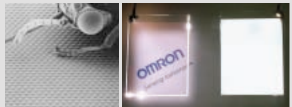
MLA Technology An array of micro-sized lenses.
